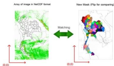
Fig 16: A comparison between the NetCDF's beginning with the beginning of the new mask image
