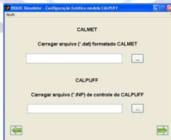
Fig. 10. Graphic Interface to inform meteorological and configuration input files to CALPUFF module.
